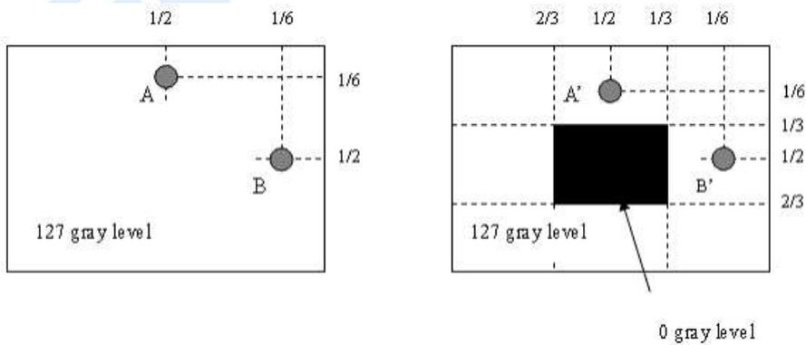
$1 \frac{LA-LA'}{LA} \times 100\% = 2\% \text{ max.}$ , LA and LA' are brightness at location A and A'.
